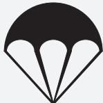
**FITTED WITH 'PARACHUTE VALVE PROTECTION'. LOAD CANNOT BE RELEASED WHEN LIFTED. ON SOME DEVICES THIS CAN BE OVERRIDDEN IN SPECIAL CIRCUMSTANCES BY OPERATING A VALVE ON THE DEVICE (USUALLY SECURED IN THE SAFE POSITION WITH A PADLOCK).**
