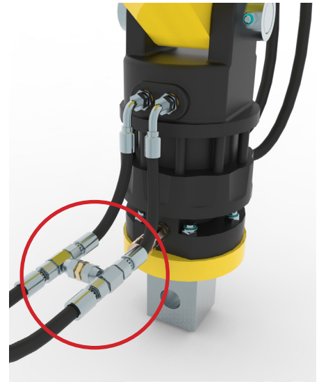
Rotator hoses are connected together using a small bore fitting to dampen out shock loadings
