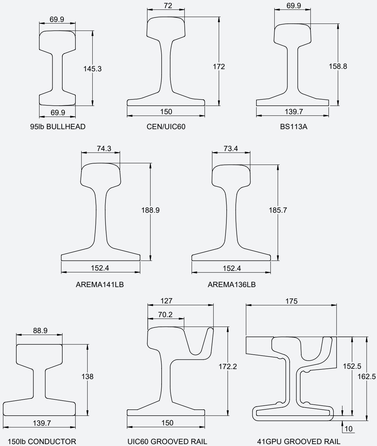
More than 50 different rail cross sections are in use throughout the world and Thomson Engineering Design Rail Handling products can be specified to suit almost any of them. The rails detailed above however are by far the most common types found in Europe and America. Most of our products will handle one or more of these rail types as standard.
