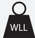
WORKING LOAD LIMIT - THE MAXIMUM RATED LOAD TO BE LIFTED BY THE DEVICE
