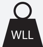
MAXIMUM RATED LOAD TO BE LIFTED BY THE DEVICE
